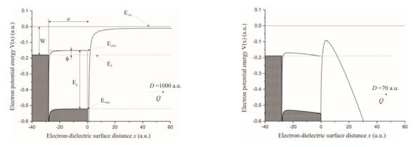
The electron potential energy inside metal Co, inside dielectric Al<sub>2</sub>O<sub>3</sub> and between the dielectric surface and ion charge Q = 44 for a) D = 1000 a.u. and b) D = 70 a.u.
